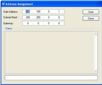
Once the TCP/IP settings are set, the web-based configuration interface of the ION-R100 can be launched from the ICT or directly in your web browser by typing the device's IP address in the address bar.
