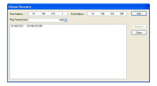
To configure Unicast Discovery, add one or more IP address ranges. Unicast Discovery will attempt to reach a device at a specific IP address in the configured ranges. Discovery can be a long process if the range of IP addresses is large. To accelerate the discovery, add several small ranges of IP addresses.
