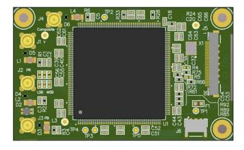
The input signal to be used by the ATOMAS-IOT-DUAL HD component breakout board is software configurable (analog SD composite or analog HD component). Only one input signal type can be used at a time.
